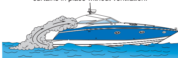
Operating with canvas tops and side curtains in place without ventilation.
