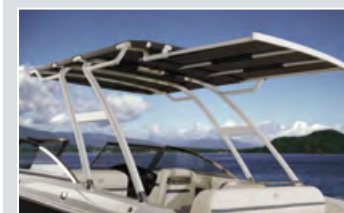
A permanent rigid structure with a stretched canvas top covering, and the extendable sunshade aft. Available for models 23SC and 25SC.
