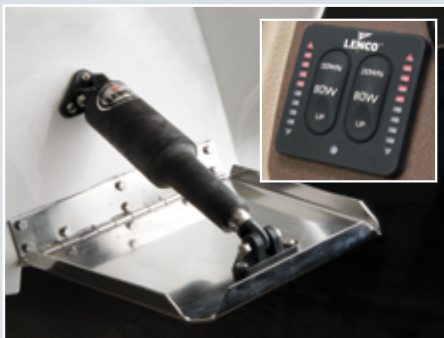
Trim Tabs - With indicators, optional Auto-Glide System available on boats 30 foot and larger.
