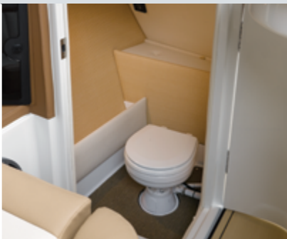
Electric Porcelain Head - Utilizes raw water drawn from thru-hull system. Shown in 25SC
