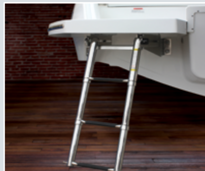
Port Boarding Ladder - 3 step telescoping ladder mount underneath swim platform.
