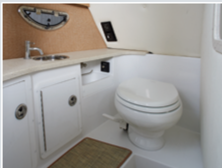
VaccuFlush Head - Utilizes water from internal freshwater system. Shown in 30SC
