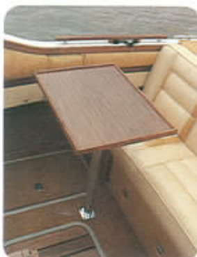
The aft dining table is supported by a polished, aluminum post. Mounting stand is through-bolted to the floor for strength and stability.
