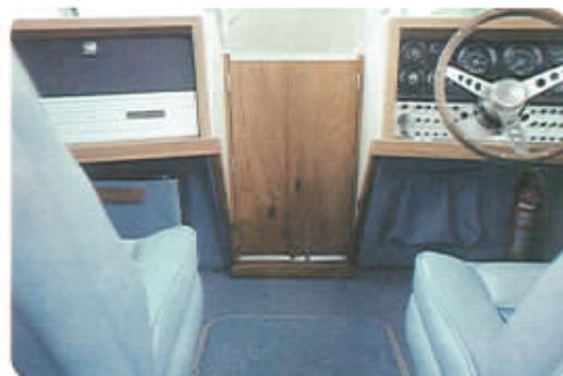
Hand crafted of solid teakwood, walk-thru doors between the open bow and the cockpit are triple hinged. A bolt latch at the bottom keeps doors securely closed and friction latches keep both doors in the open position.
