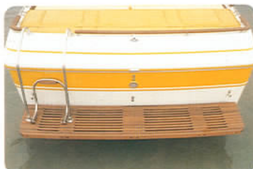
Solid teakwood, doweled and marine glued, the swim platform has been tested to withstand 800 pounds of force. Swim platform with middle section hinged is available for single engine models and full single unit platform for twin models.
