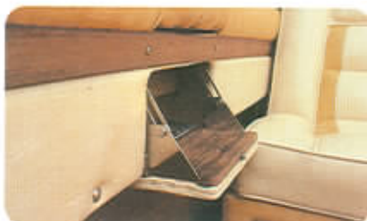
Aft boarding steps are hand crafted of grooved teak and stainless steel. It conveniently folds into the side wall when not in use.
