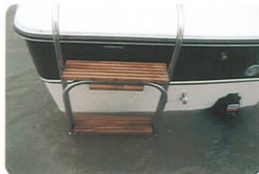
Boarding ladder with fold down step is constructed of stainless steel with teak steps. Steps are grooved to prevent slipping. Locking latch secures fold down step in upright position.
