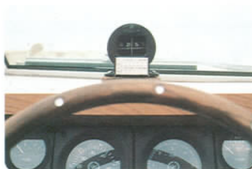
Directional navigation is enhanced with the addition of this precisely, accurate compass. A luminous dial allows night reading. Centrally mounted on instrument panel frame. (Bow Rider models only)
