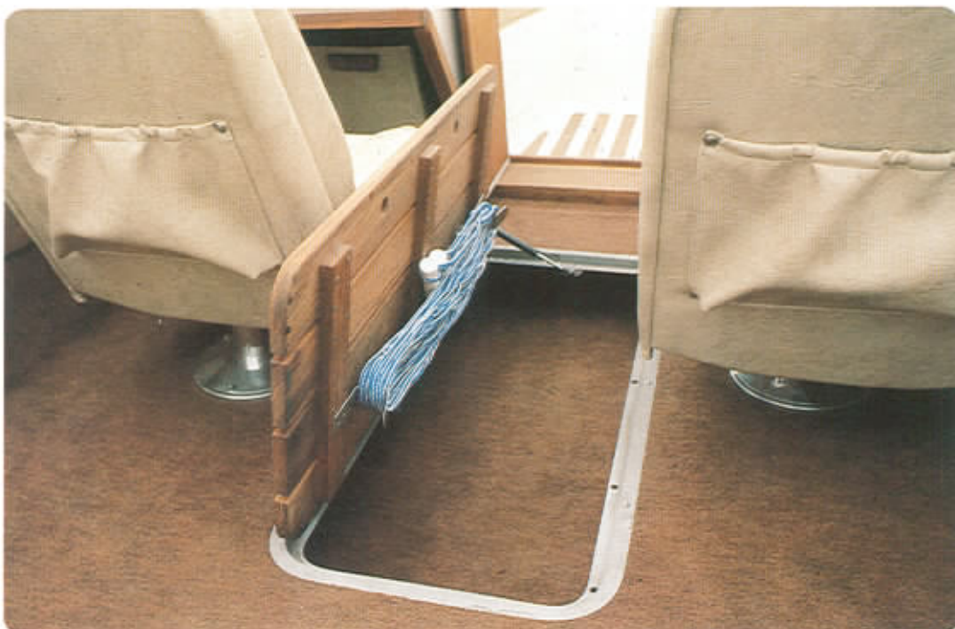
Carpeted, spacious ski storage compartment provides room for several pairs of skis. The solid teak hatch is smoothly opened and closed with the aid of a counter-balance-assist cylinder. Mounted on the hatch, stainless steel line wraps provide neat ski rope storage.
