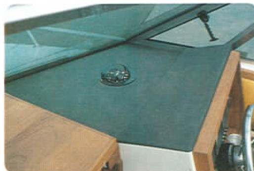
Directional navigation is provided with this 5", illuminated dial compass. Contains double axis gimbal systems and sapphire jewels for maximum accuracy and dependability.
