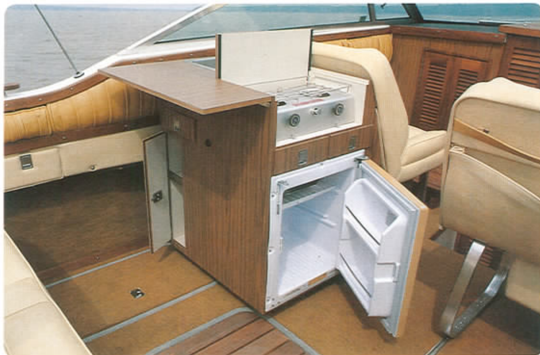
Elegant chef's galley has all the necessities for small, meal preparation: a twelve volt, two cubic foot refrigerator; two burner alcohol stove with protective cover; stainless steel sink with demand water pump (two five gallon storage tanks are located under the passenger's seat) and a fold-out preparation table complete this compact galley.
