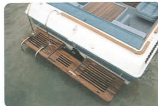
Dowel pinned and marine glued, this solid, teakwood swim platform has been tested to withstand up to 800 pounds of pressure. Center section is stainless steel hinged for upward movement when outdrive is up.
