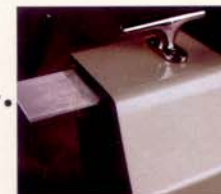
Hardware secured to aluminum plates embedded in fiberglass for maximum strength.
