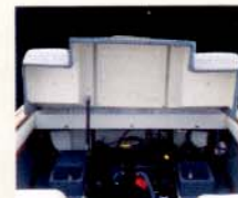
One-piece fiberglass motor box provides easy access to engine compartment.
