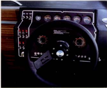
Glare-resistant, flat black anodized aluminum dash panel with full instrumentation.
