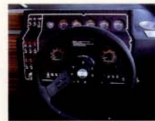
Flat black anodized aluminum dash panel for glare resistance and maximum durability.
