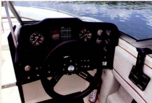
Dart system in-dash computer available on 202 and 202SE, and VDO instrumentation available on 202, 222 and 223.
