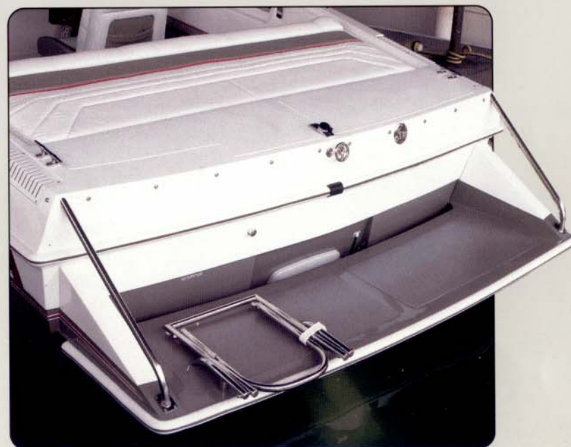
192 Fiberglass swim platform with fold down step
