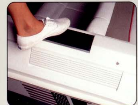
Molded-in boarding step with rubber insert (202/203)
