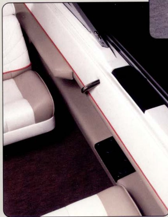
Molded-in boarding step and rear passenger hand hold (202/203)
