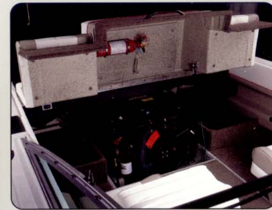
Motor box raised (Shows optional halon fire control system)
