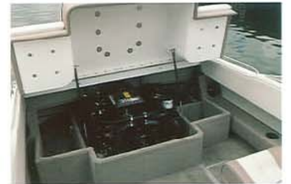
One piece fiberglass motor box adds to longevity and serviceability.
