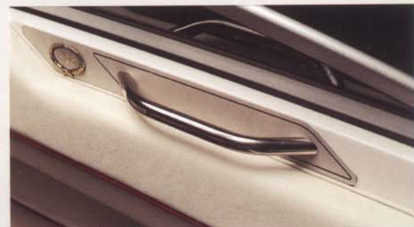
Stainless grab rails are mounted to 1/4" backing plates in the fiberglass.
