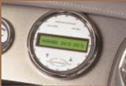
Perfect Pass Wake Board Pro Cruiser Control (replaces tach)
