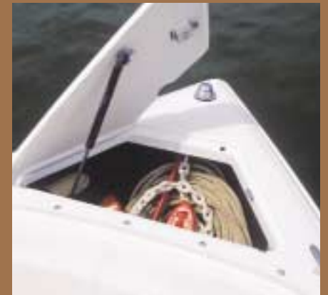
Anchor Locker with Gas Assists Cylinder
