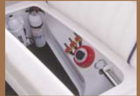
Bench Seat Storage and Battery Switch
