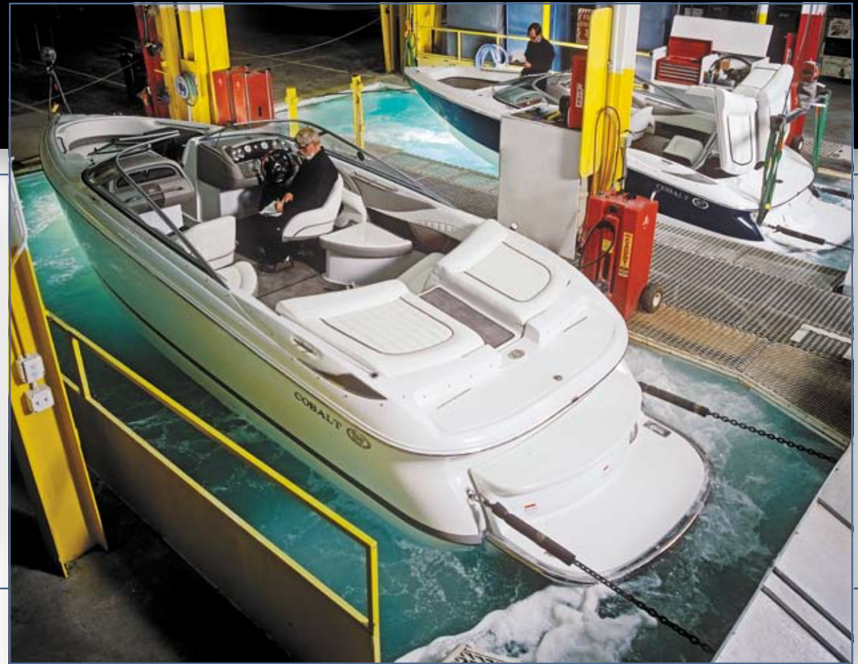
Every boat produced is put through a 30-point check while run under load for 30 minutes in the test tank.
