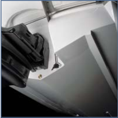
The extended running surface provides quicker planing, firm and true turns, minimized bow rise, and enhanced lift astern.
