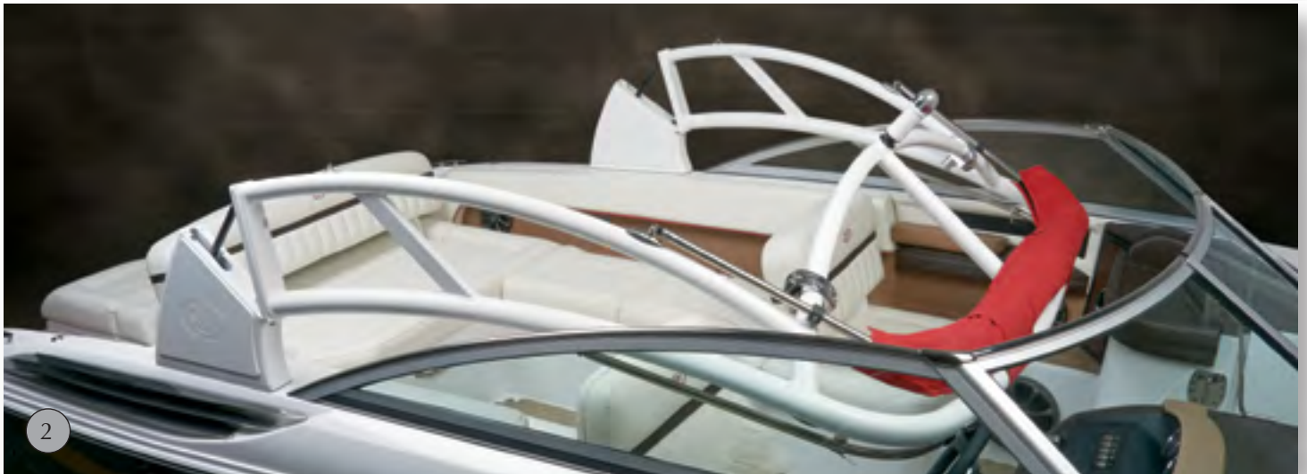
2. Aluminum Forward Folding Arch with Bimini folds easily with manual gas assist cylinders or by electric actuators.
