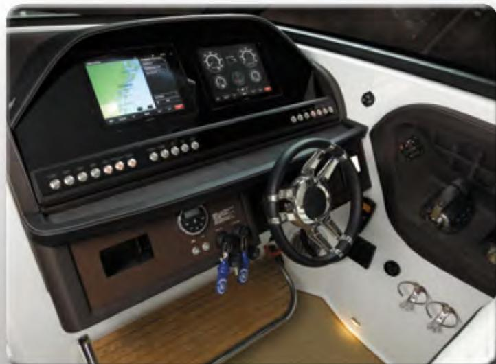
Glass cockpit design allows for multiple configurations of displays. GPS, available radar, tide charts, and engine data can be easily accessed.
