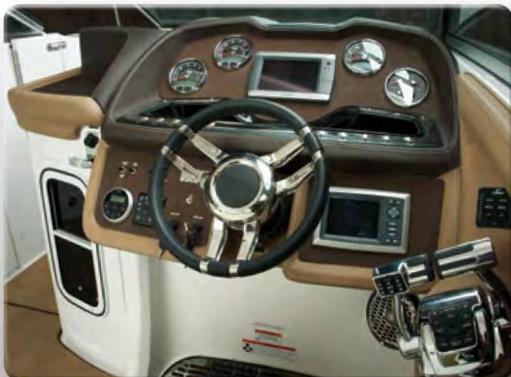
Helm station with full digital instrumentation, in-dash GPS, engine systems display, and (DTS) digital throttle and shift.
