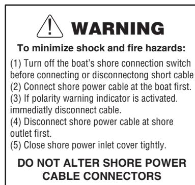
Shore Power Connection
