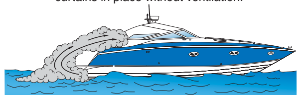
Operating with canvas tops and side curtains in place without ventilation.
